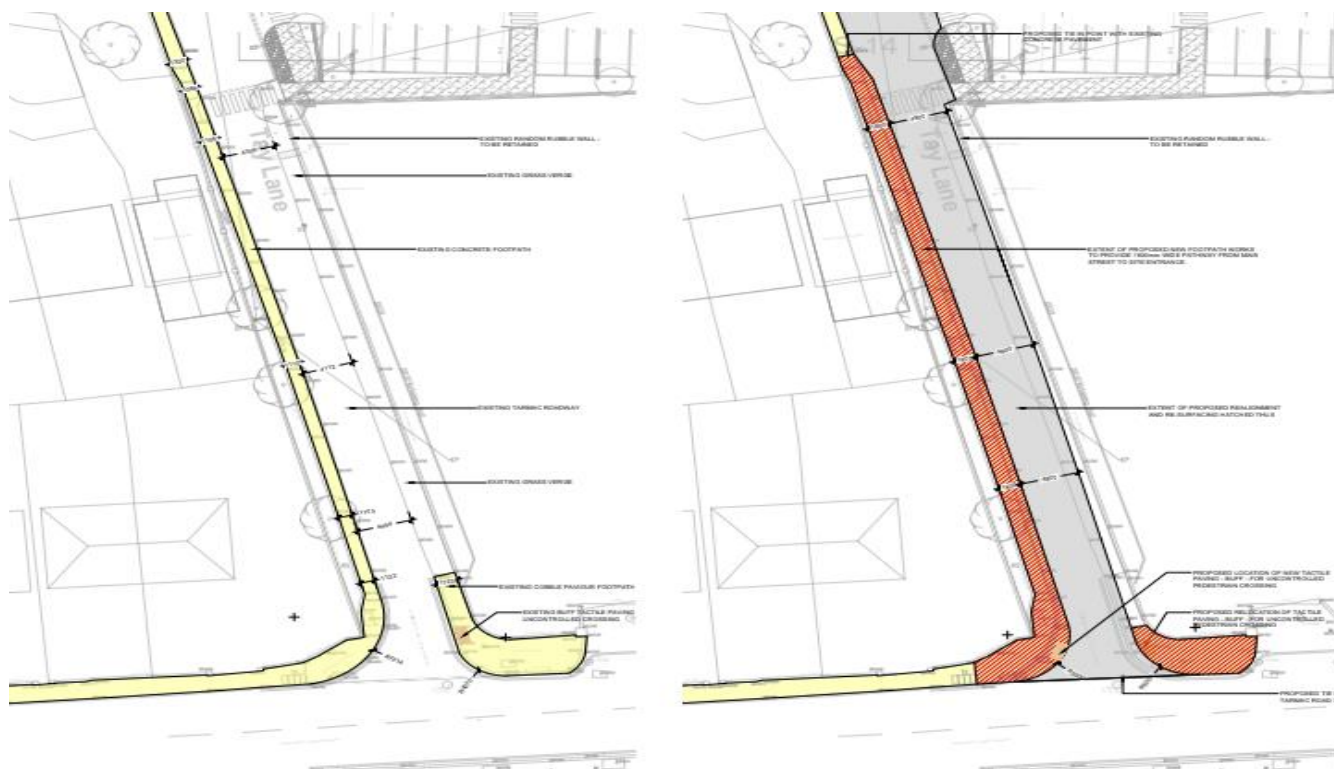
Figure 12.0 Excerpt from 'Existing and Proposed Laneway Layout' drawing showing the proposed improvements to Tay Lane.
