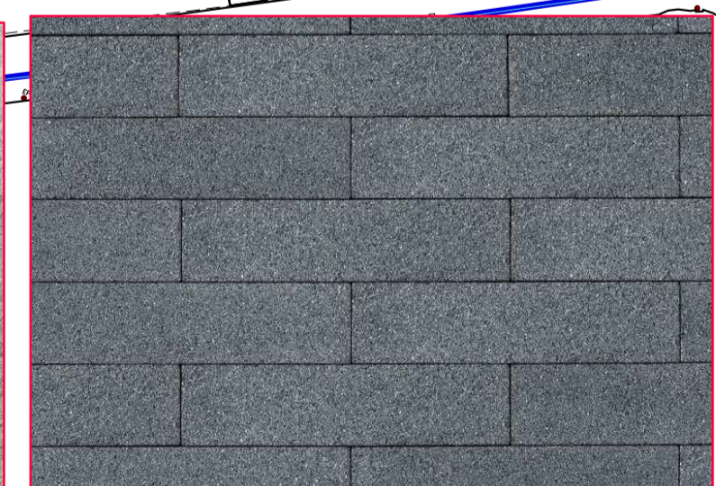
Natural granite aggregate paving, graphite finish. 600mm x 150mm x 80mm depth.
