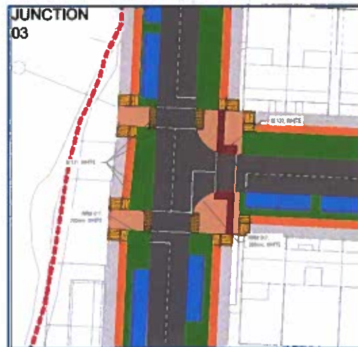
Figure 2-6 - Signalised Junction No. 2
