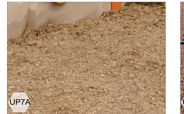
UP7A - Engineered Woodchip Surfacing NOTE: Grass Berm to enclose Woodchip surface. See Section A-a for interaction with Tiger Mulch Surfacing.
