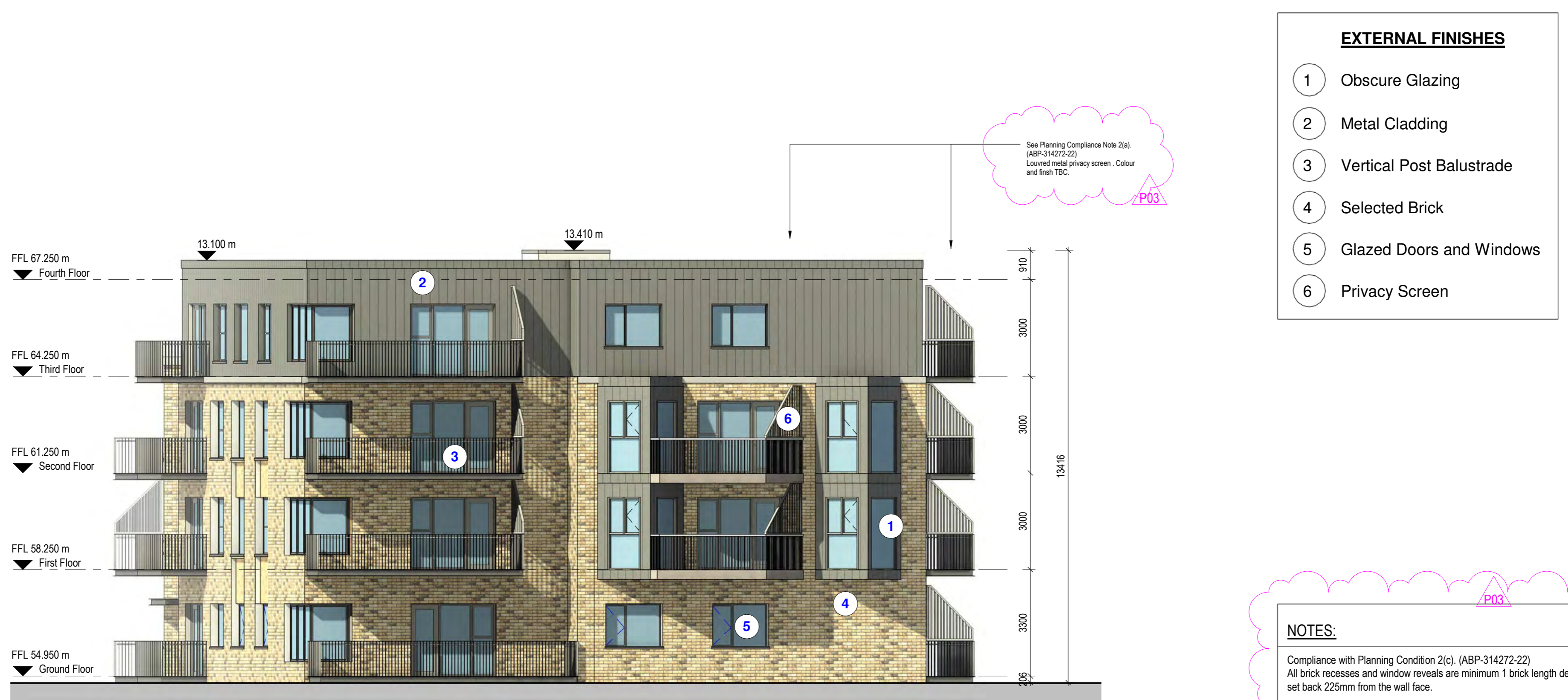
BLOCK 3 EAST ELEVATION FACING BLOCK 2 1 : 100
