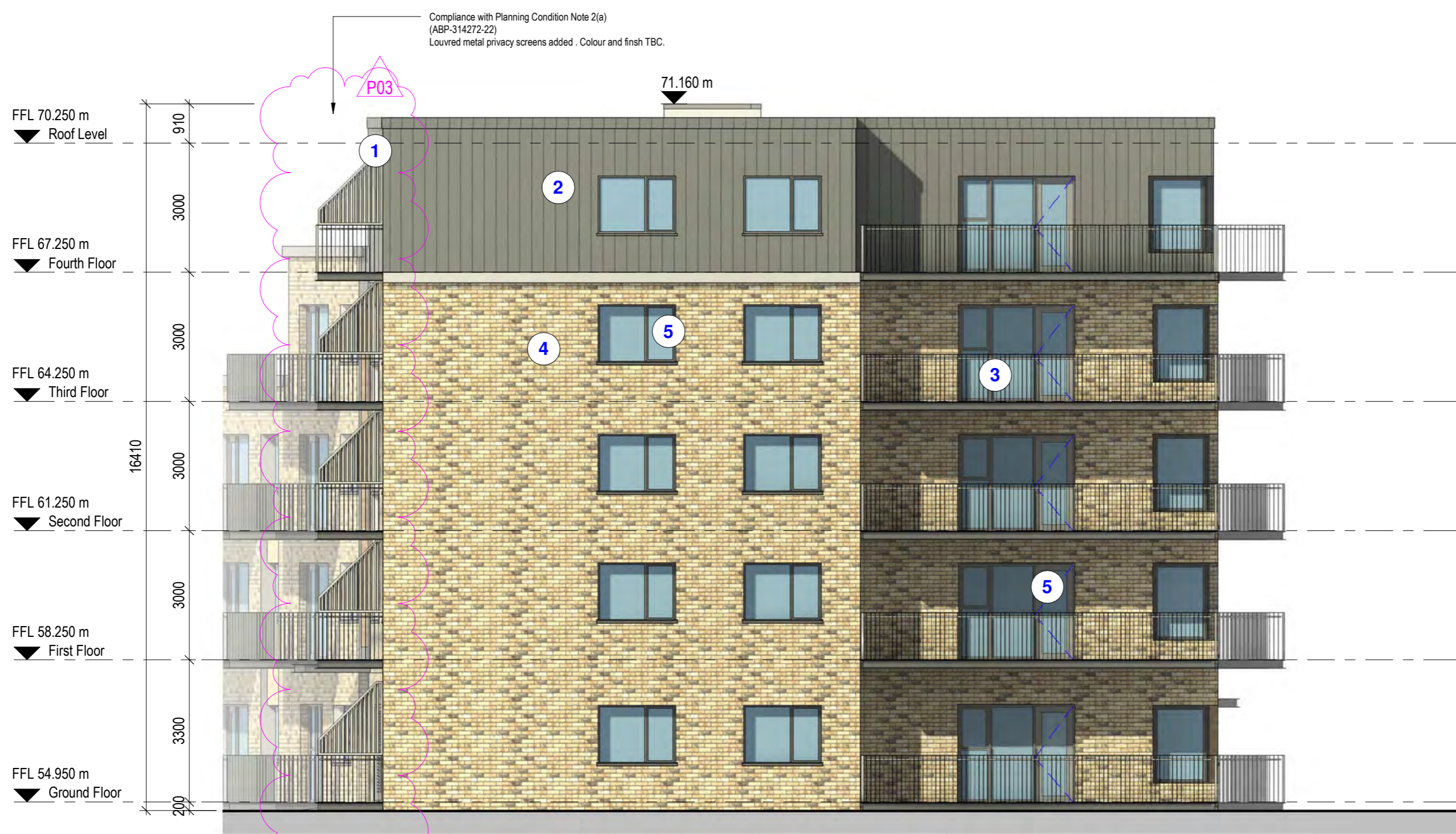
BLOCK 2 SOUTH ELEVATION FACING BLOCK 3 1 : 100
