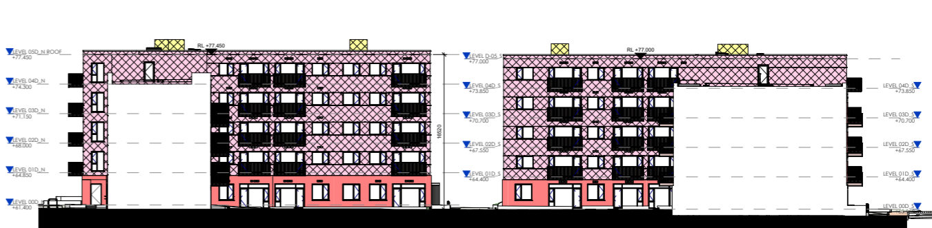
4 BLOCK D - EXTERNAL WALL TYPES - WEST COURTYARD 1 : 200
