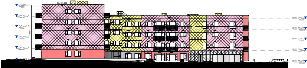
1 BLOCK D - EXTERNAL WALL TYPES - NORTH COURTYARD 1 : 200
