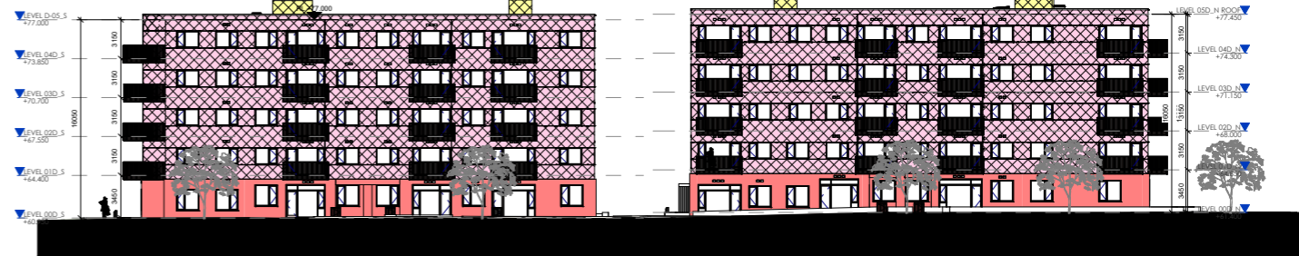
3 BLOCK D - EXTERNAL WALL TYPES - EAST 1 : 200
