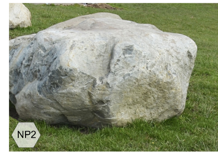
NP2; Locally Sourced Glacial boulders - various sizes upto 300 - 600mm high Installation; 300mm below ground, Form; Rounded edges
