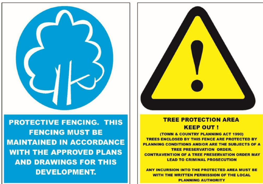
Figure 5.8 Signage to be erected on RPZ fencing
