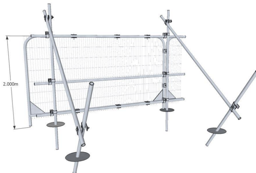
Figure 1. Protective fence specification
