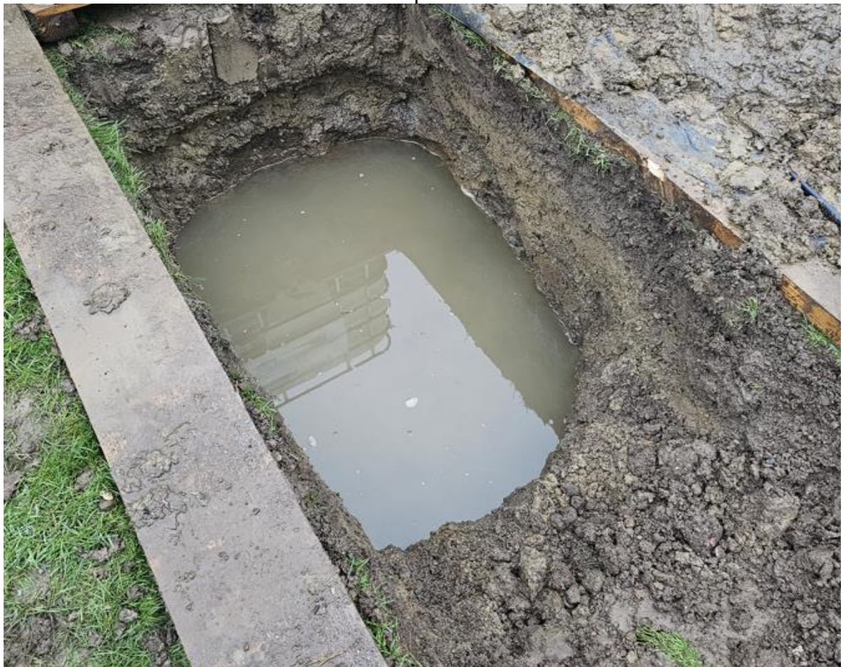
Trial Pit 24 hours after excavation – Depth 1.6 settled water level at 0.7m
