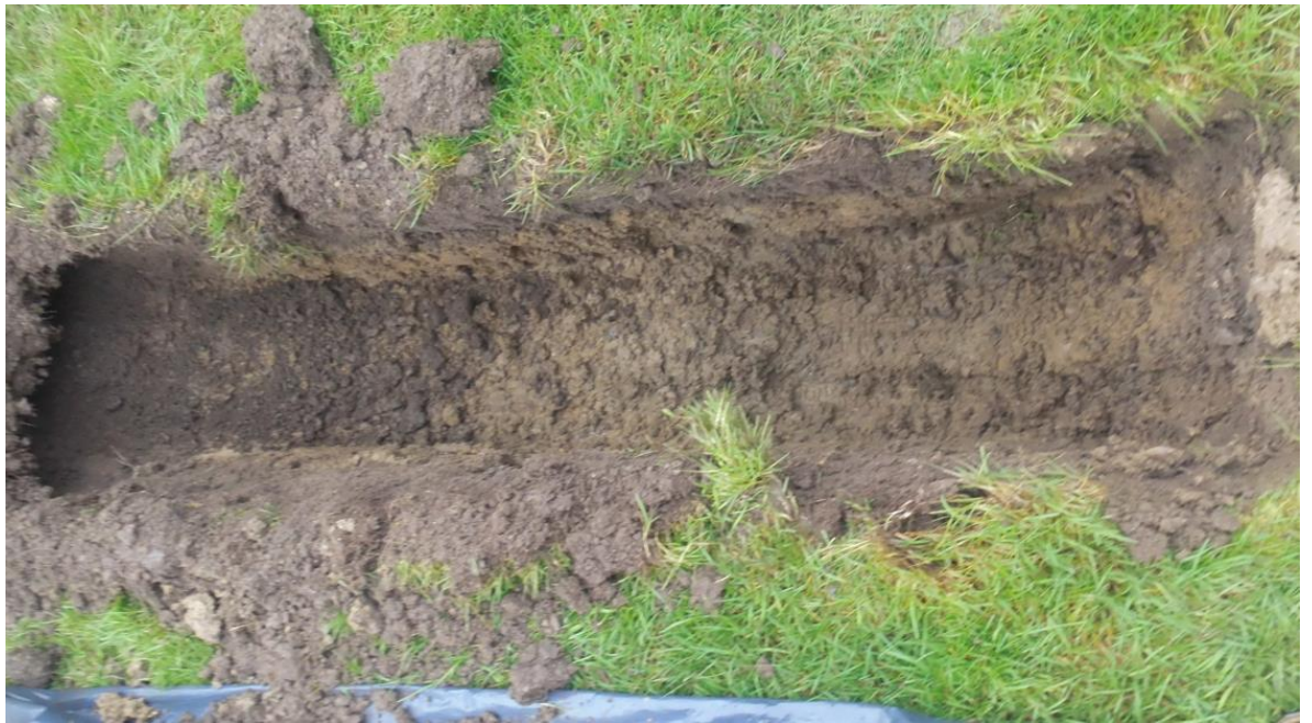
Test Pit before water added – Depth 0.6m from original ground level
