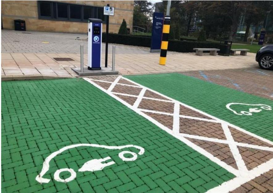
*Figure 3 - Proposed EV car charging space road markings*
