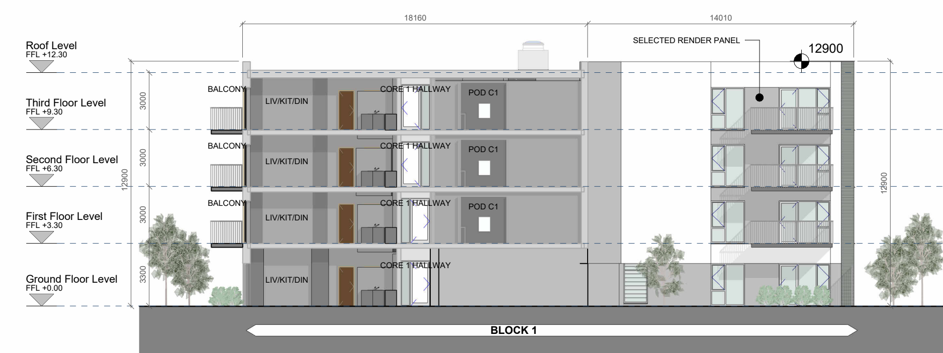
5 Block 1 - South Courtyard Elevation SCALE: 1 : 200
