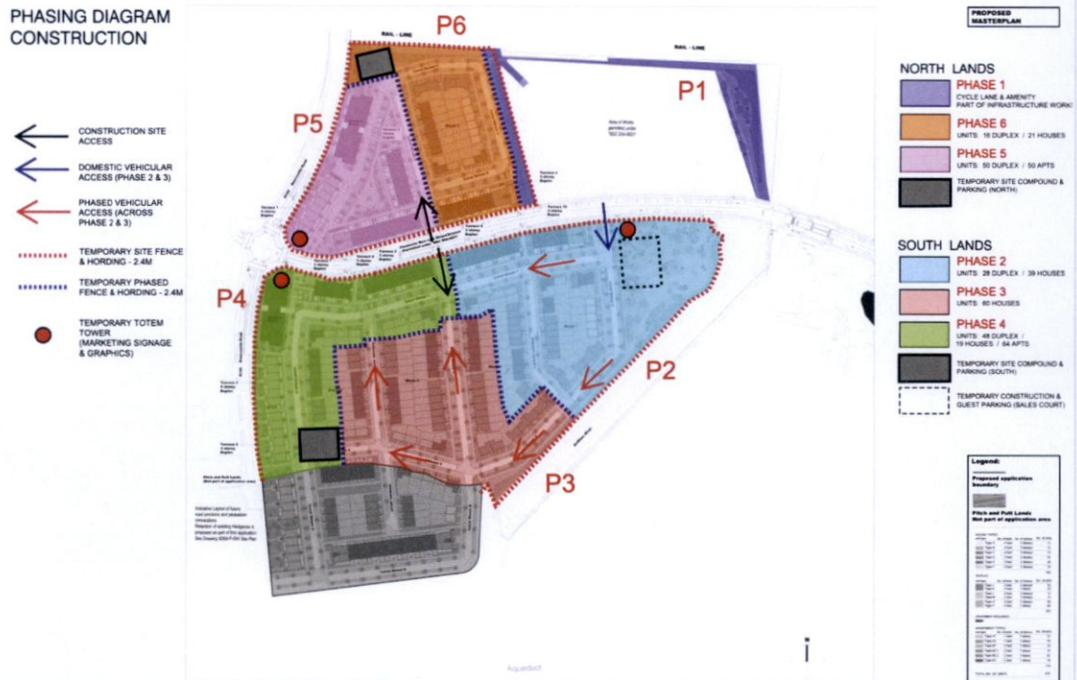
Figure 5: Extract from the Construction & Environmental Management Plan, prepared by AWN Consulting showing the proposed construction phasing of the proposed development.
