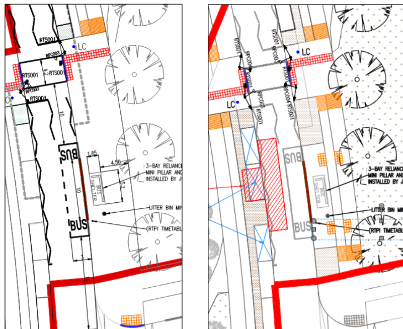
Figure 3: Comparison between previous (left) and current (right) design for pedestrian footpath and cycle track behind bus stop
