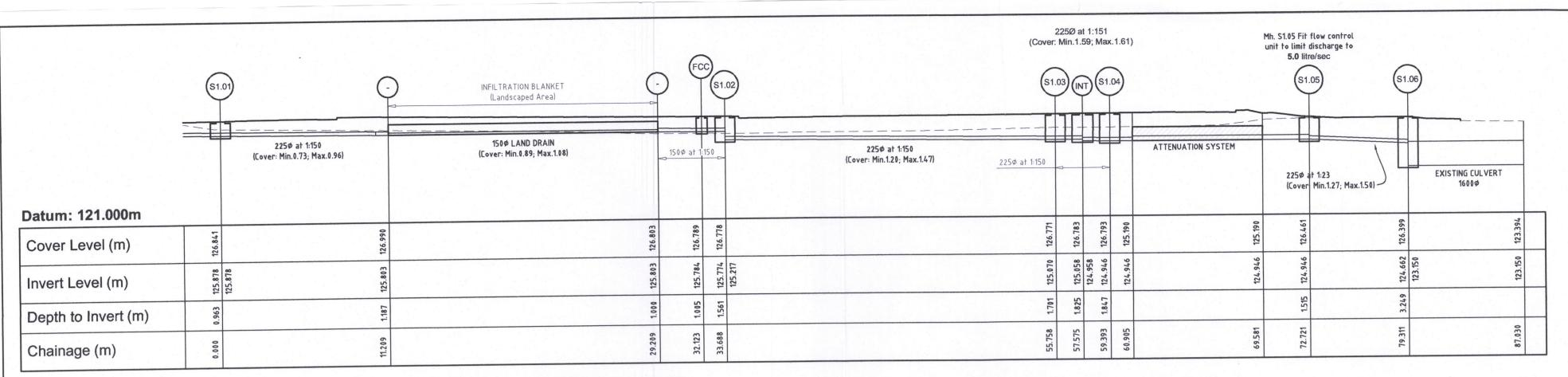
Surface Water Drainage - Longitudinal Section (S1.01 to Existing Culvert)
