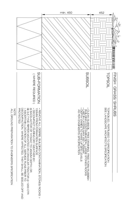
Detail D 01 Drawing LD-04-CS Topsoil depths and Bark Mulch specification to planted areas Scale @ 1:20
