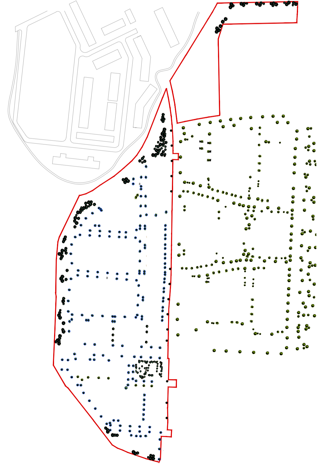
Proposed new street trees 193 no. Proposed new open space trees 219no. Proposed bio retention tree pits 187 no. Proposed swales, total length 138 linear meters. Proposed Street trees to Cellbridge link road as per SDZ 17A/0009;14no.
