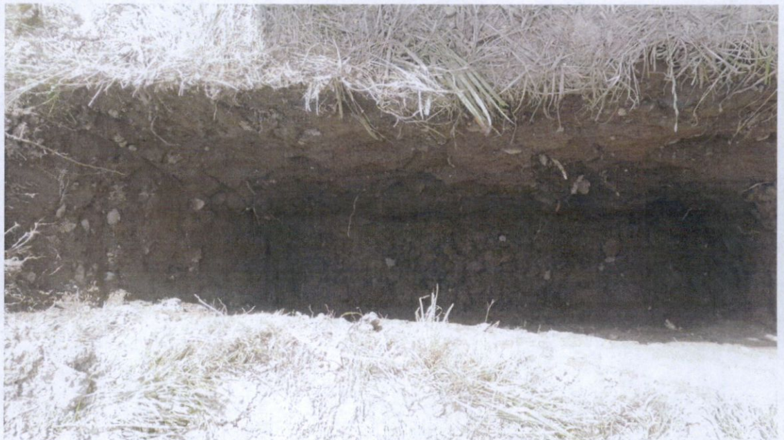
Test Pit before water added – Depth 1.0m
