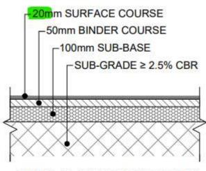
DETAIL B: ASPHALT FOOTPATH DETAIL (1:20)
