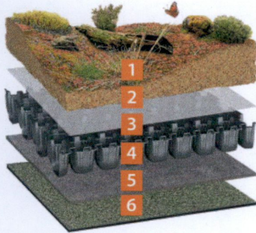
Figure 7. Bauder visualisation showing a build-up of semi-intensive bio-diverse green roof with a 150-200mm undulating growing medium, planted with plug plants, and occupied with biodiversity features such as dead logs and piles of stones and sand
