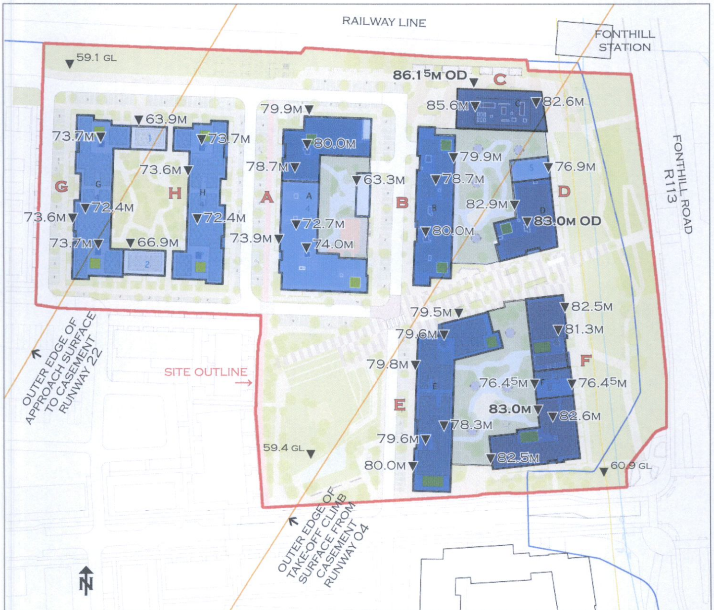
SITE PLAN OF PROPOSED DEVELOPMENT WITH ELEVATIONS (O.D.) OF HIGHEST PARTS SCALE 1:1,750 APPROX. [AT A4 SIZE]
