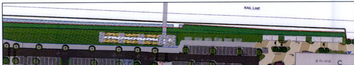
Updated layout – Planning RFI – shows that the path has been narrowed to the minimum for a shared path and additional planting included where possible, as well as reinforced grass for cycle parking spaces.
