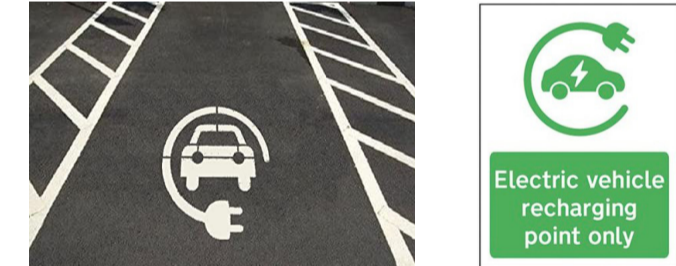
PAINTED CAR PARK BAY SYMBOL, 740x810mm WHITE OR GREEN PAINT TO LOCAL CO. CO. STANDARDS ELECTRIC VEHICLE RECHARGING POINT ONLY- 30MM ALUMINIUM-DIBOND SIGN 300MM X 200MM MOUNTED ON STANDARD NRA SPEC POLE FOR PRIVATE ROADS ONLY
