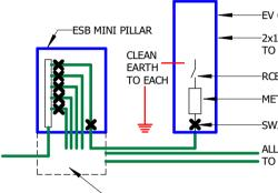
—2x11kw 5c 10sqmm SWA/LSZH TO EV CHARGER (35m RUN MAX) -RCBO RATED FOR EV ALL CABLES IN ESB DUCTS
