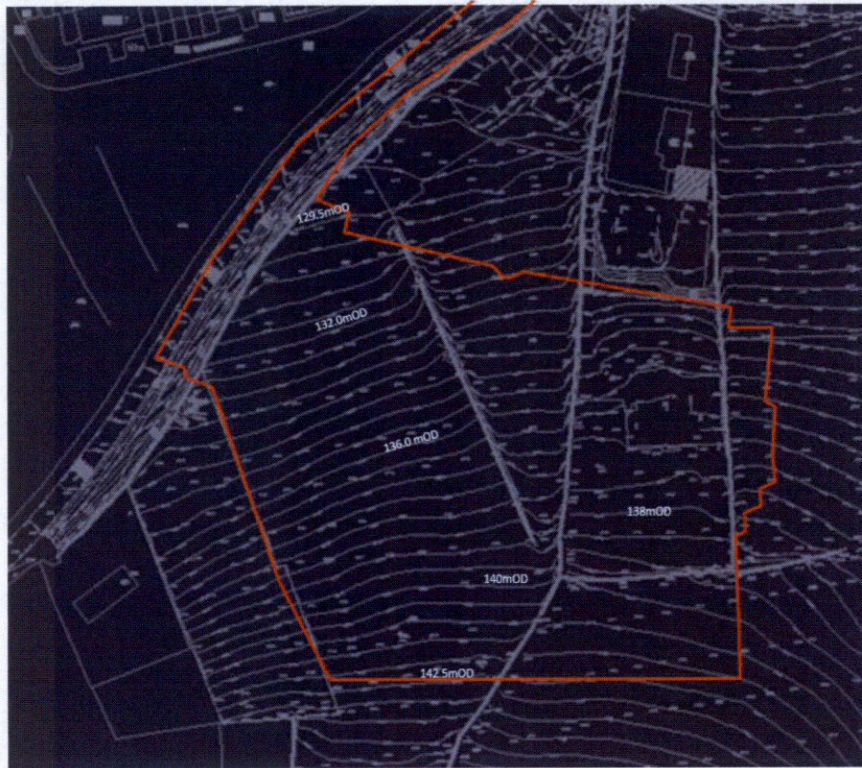
Figure 2-2: Screenshot from Topographical Survey with Annotated Spot Heights and Approximate Redline Boundary (AECOM 2023. X-Topo 2D ITM)
