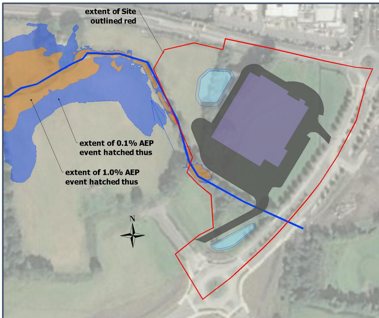
Figure 6-2 Fluvial flood risk zones - Pre-Development
