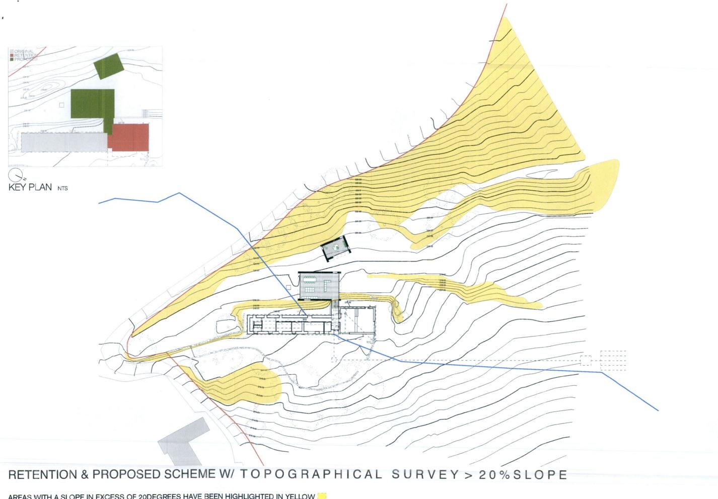
AREAS WITH A SLOPE IN EXCESS OF 20DEGREES HAVE BEEN HIGHLIGHTED IN YELLOW 100m ZONE FROM STREAMS
