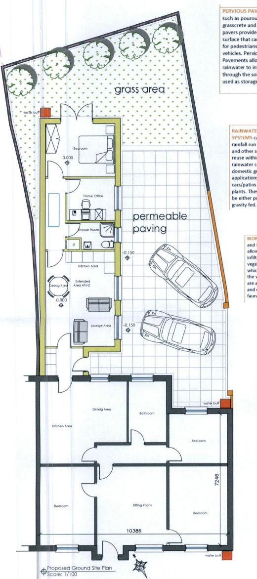
**PERVIOUS PAVEMENTS** such as pourous asphalt, grasscrete and permeable pavers provide a hard surface that can be used for pedestrians or vehicles. Pervious Pavements allow rainwater to infiltrate through the soil or can be used as storage systems.
