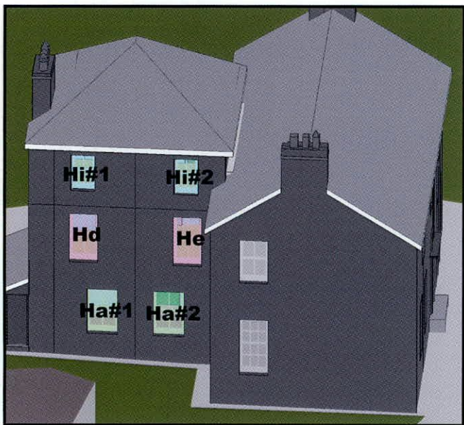
Figure 5.1: Windows/Rooms impacted for VSC.
