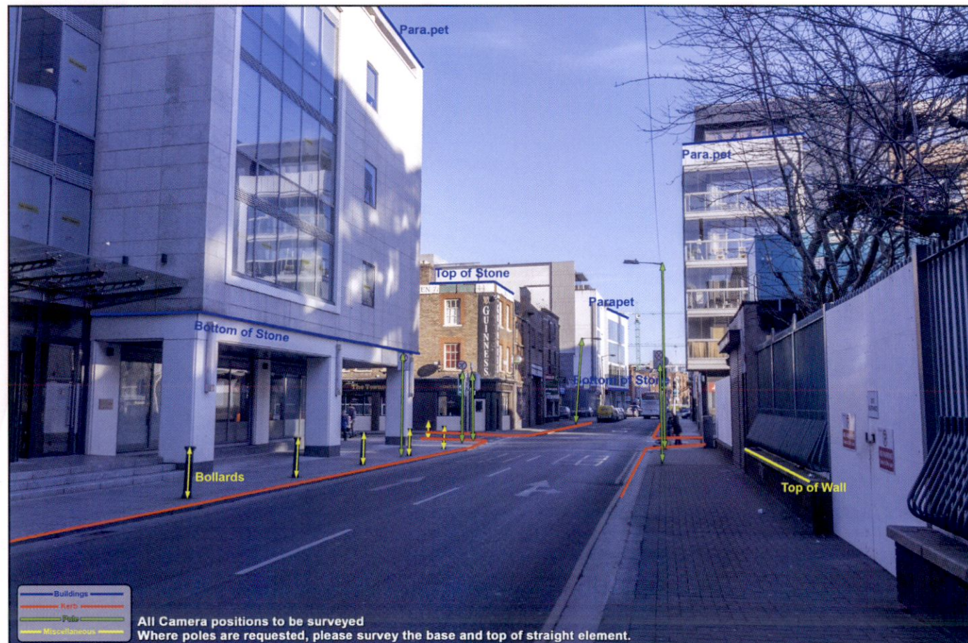
Fig.7: Fixed reference points marked for surveyour.
