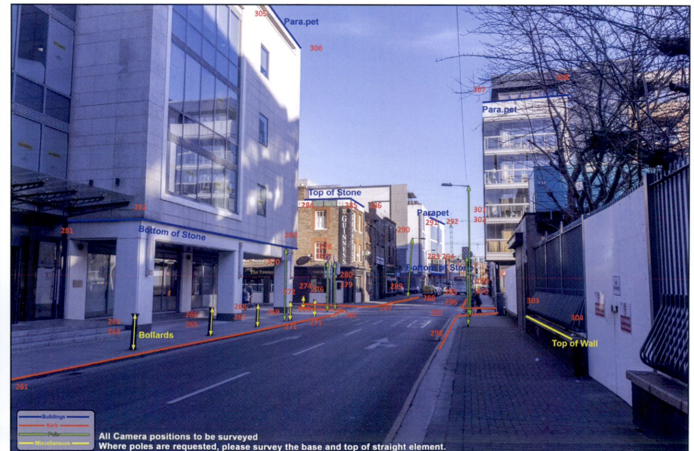
Fig.8: Fixed reference points surveyed and numbered by surveyor.
