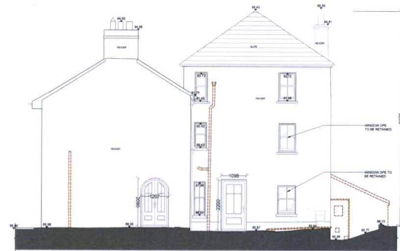
Revised Side Elevation
