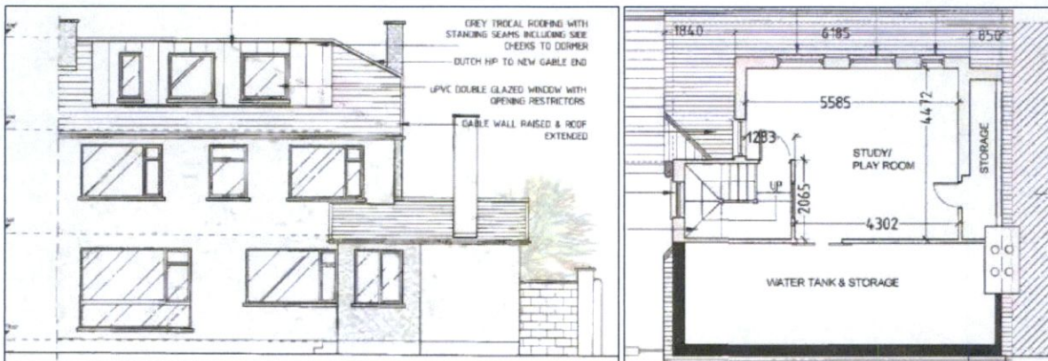
Figure 19.0 Rear elevation (l) and attic floor plan (r) granted at further information stage under Ref. SD22B/0100.
