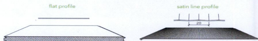
Picture 44: Composite cladding textures: flat for the proposed building, satin line (also called micro ribbed) for the generators enclosure.
