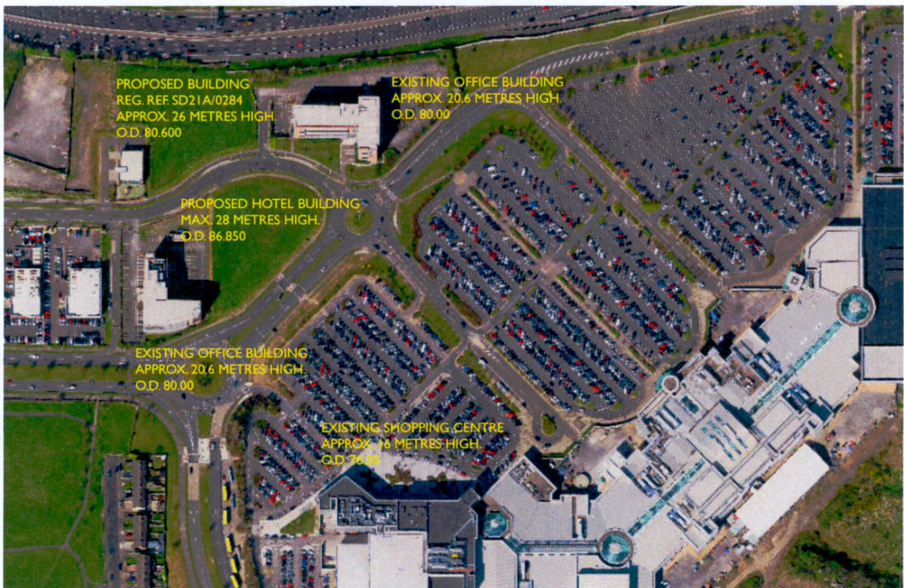
Fig. 9; Existing and proposed building heights and approx. parapet levels relative to Ordnance Datum.
