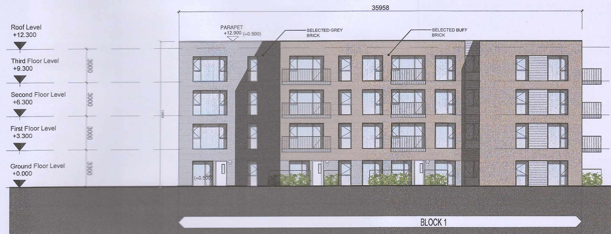
2-BLOCK 1 - NORTH ELEVATION
