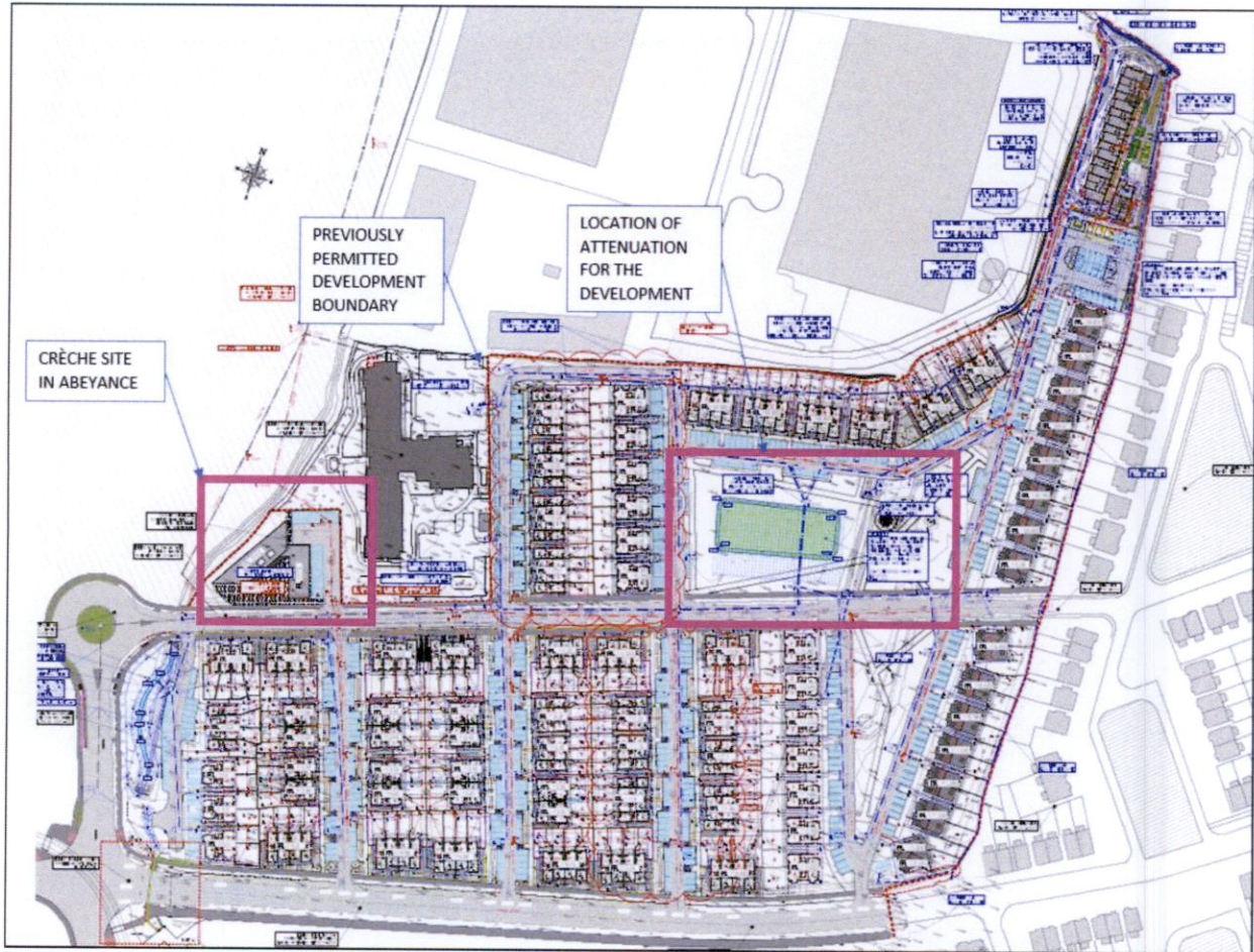
Figure 3A - 2: Extract from Surface and Foul water site layout plan – For Permitted Development
