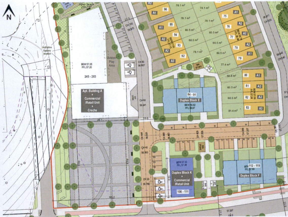
Fig. 1 – Site layout plan including urban plaza proposed at AI stage
