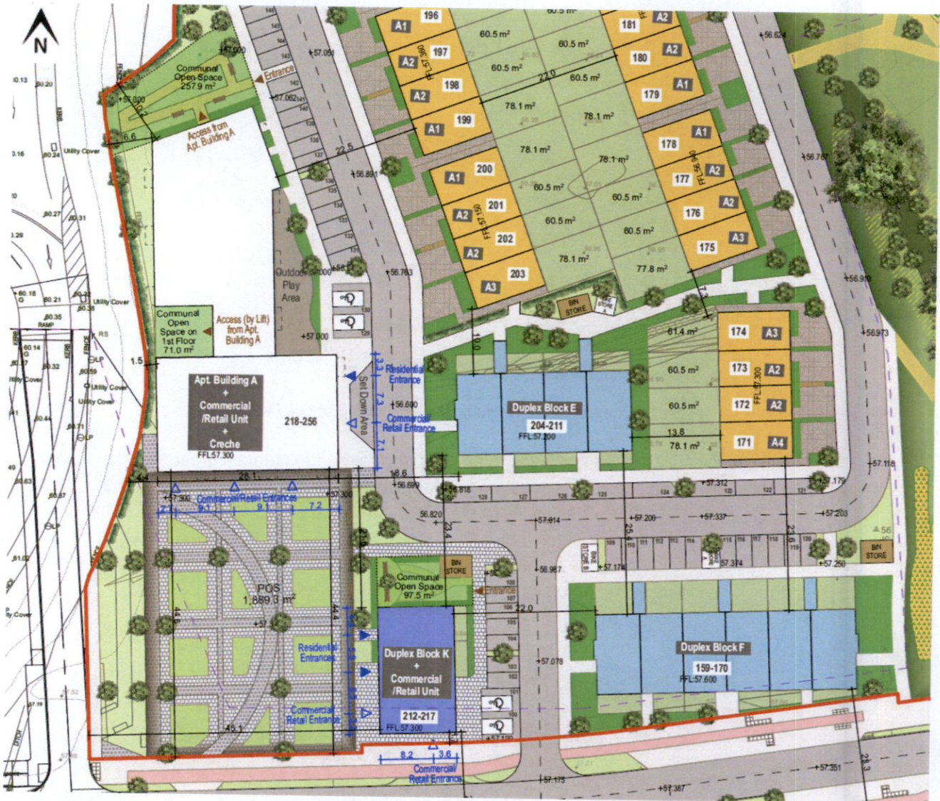
Fig. 3 – Revised proposed site layout plan including urban plaza, with Block K repositioned to enclose the plaza on its eastern side.
