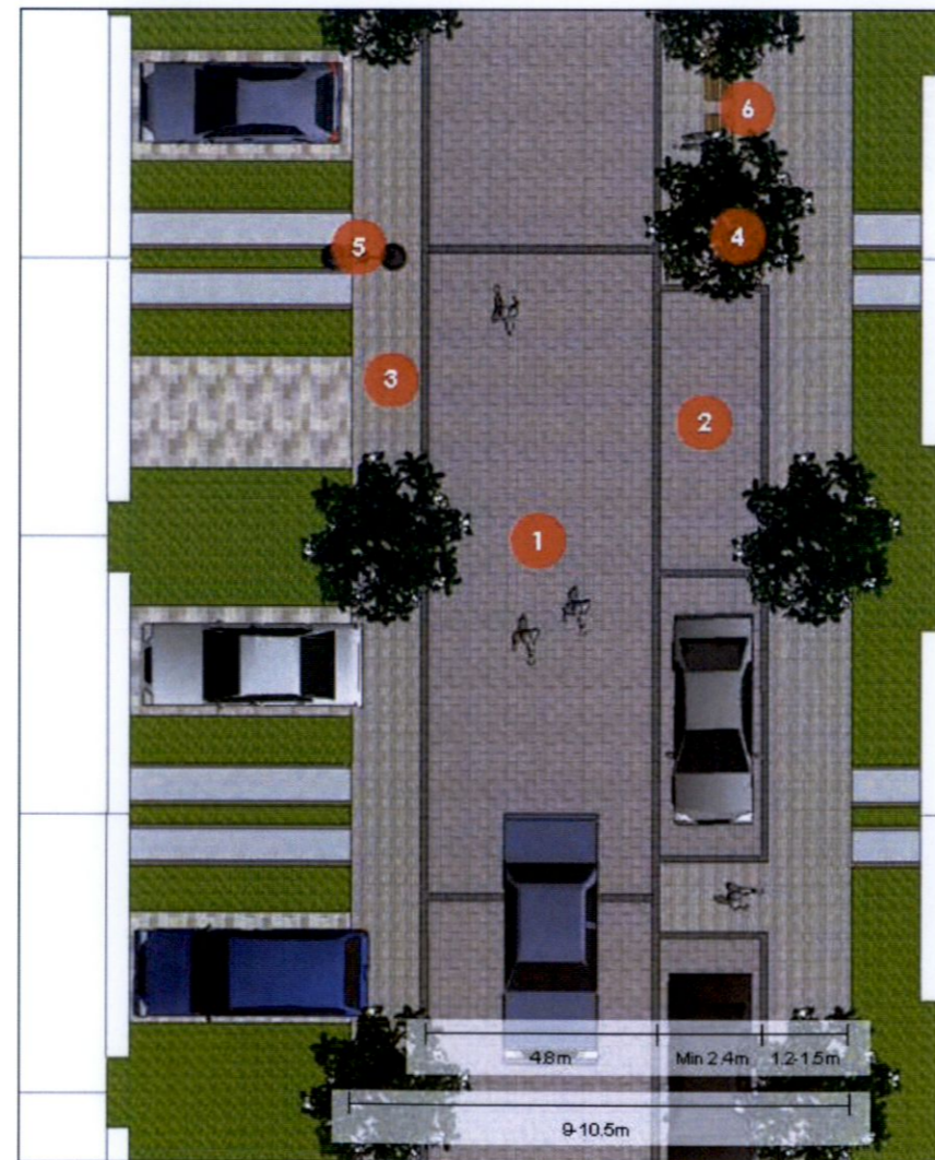
Typical treatment Back Street designated as homezone/shared surface street. For application throughout Adamstown on where suitable streets are identified.
