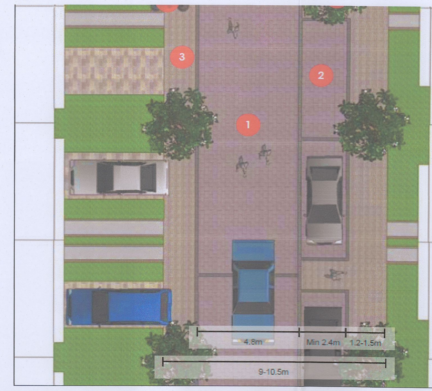
Typical treatment Back Street designated as homezone/shared surface street. For application throughout Adamstown on where suitable streets are identified.
