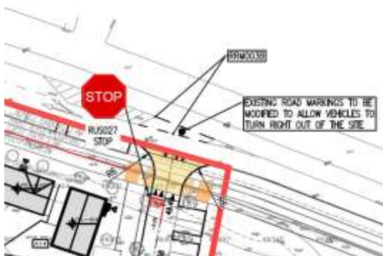
Figure 1: Junction to Adamstown Drive
