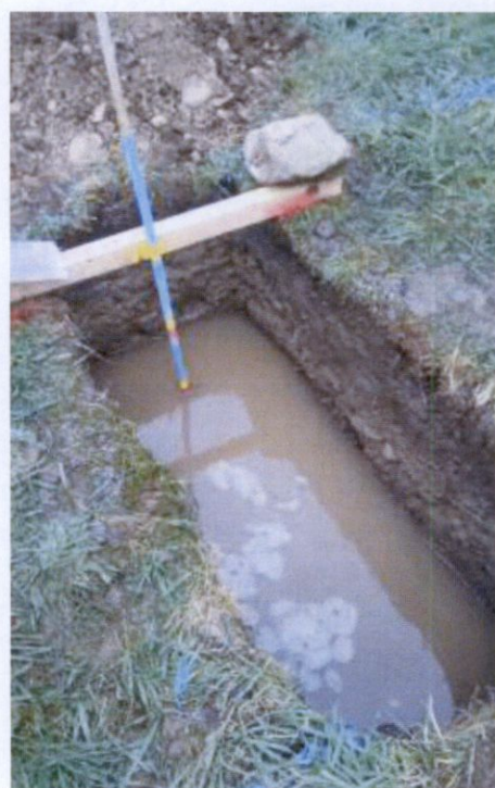
Infiltration Test in Progress
