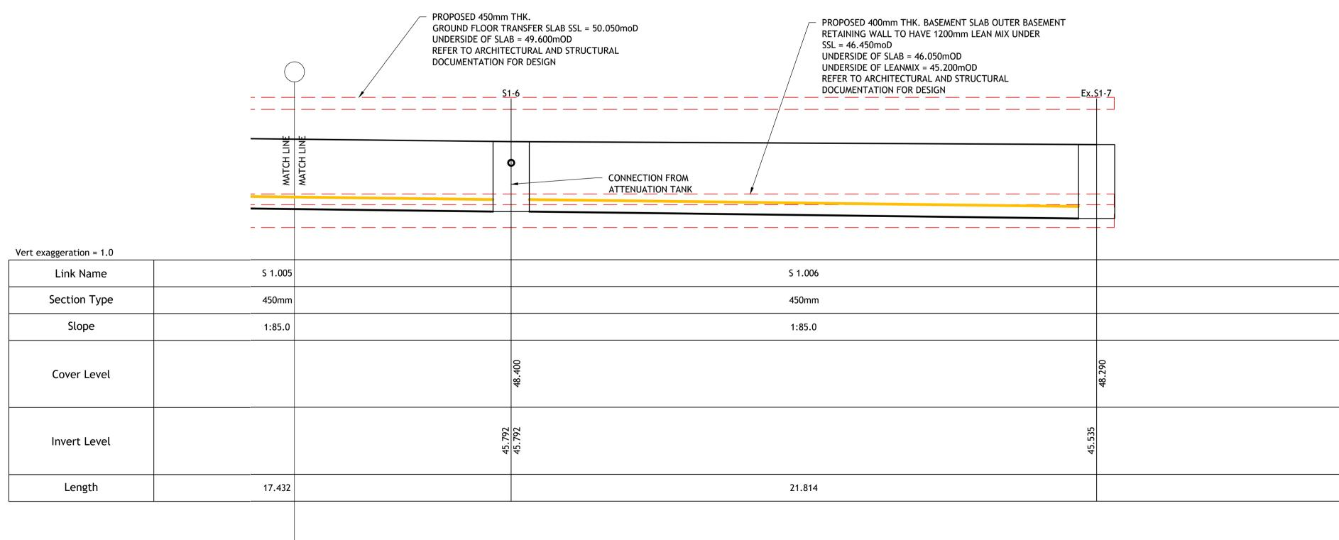
PROPOSED SURFACE WATER SEWER DIVERSION LONG SECTION (CONT.)
