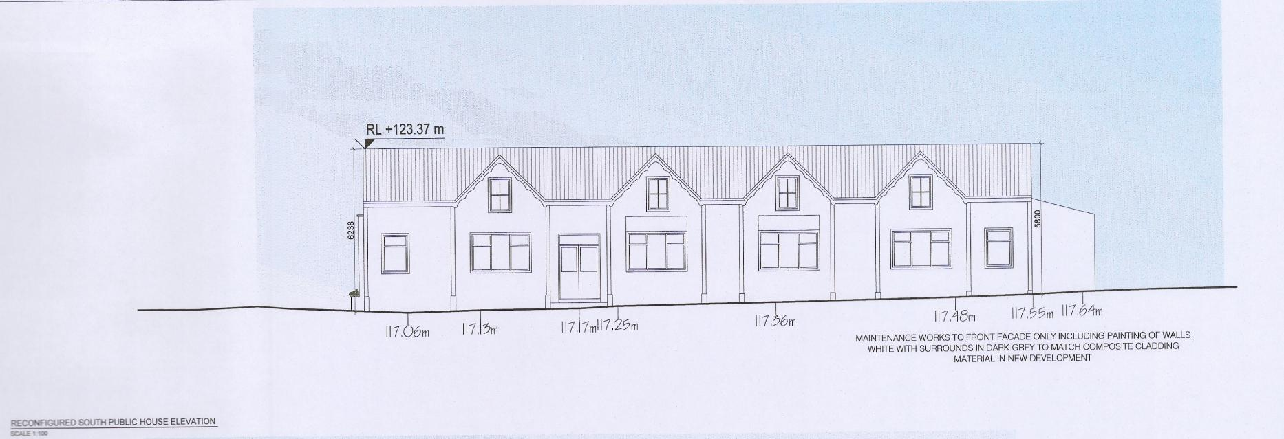
RL +123.37m RL +122.73m RL +121.95m 117.71m EXTERNAL COURTYARD STRUCTURE TO BE MAINTAINED WITH SECONDARY ACCESS TO PUB FROM PARKING AREA OF NEW PROPOSED DEVELOPMENT YARD FOR PUB PROPOSED FOR THIS LOCATION ADJACENT SECONDARY ACCESS TO PUB EXISTING ENTRANCE TO BE BLOCKED UP AND PAINTED TO MATCH THE ADJOINING
