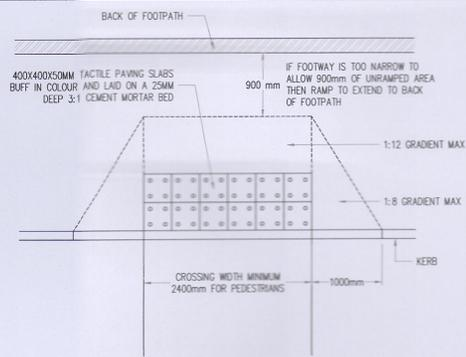
**TACTILE PAVING PLAN AT UNCONTROLLED PEDESTRIAN CROSSINGS.**
