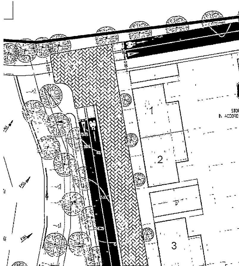
Figure 2 – Cul de Sac Turnaround Area
