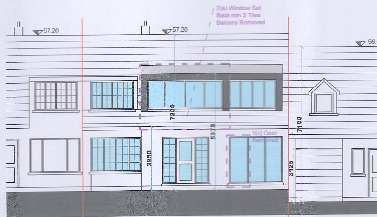
Proposed Front Elevation (East) Scale 1:100
