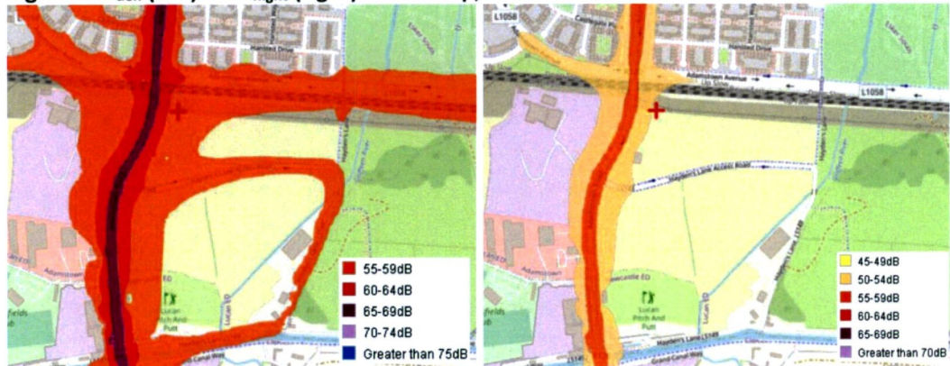
Figure 7: L_{den} (left) and L_{night} (right) Noise Map, Round 3: Road Sources
