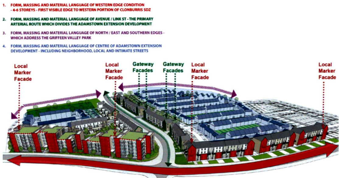
Figure 20: Extract from the Design Rationale, prepared by Burke Kennedy showing how the height, form, massing and materiality reflect to the different conditions of the Adamstown Extension Development Area.
