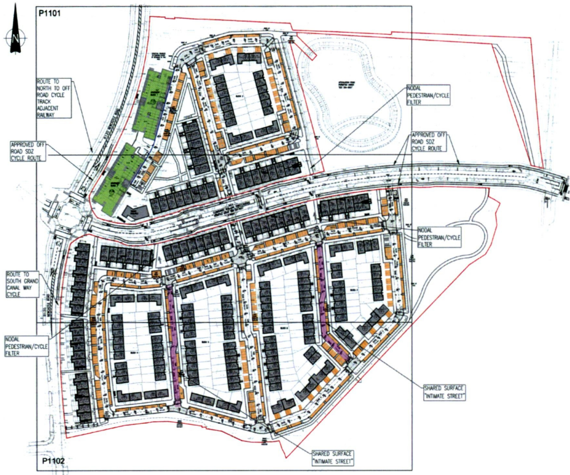
Figure 17: Extract from Dwg. No. 21-055-P1100 Road General Arrangement, prepared by Waterman Moylan Consulting Engineers showing the proposed road alignments.
