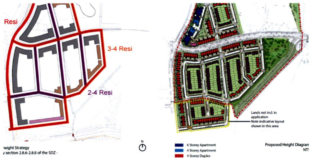
Figure 22: Extract from the Design Rationale, prepared by Burke Kennedy showing how the proposed building height aligns with the provisions of the Planning Scheme.
