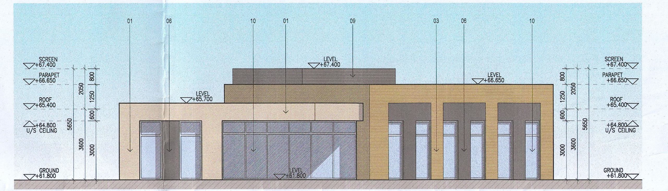
05 Amenity Building - South-West elevation 1:100 @ A0
