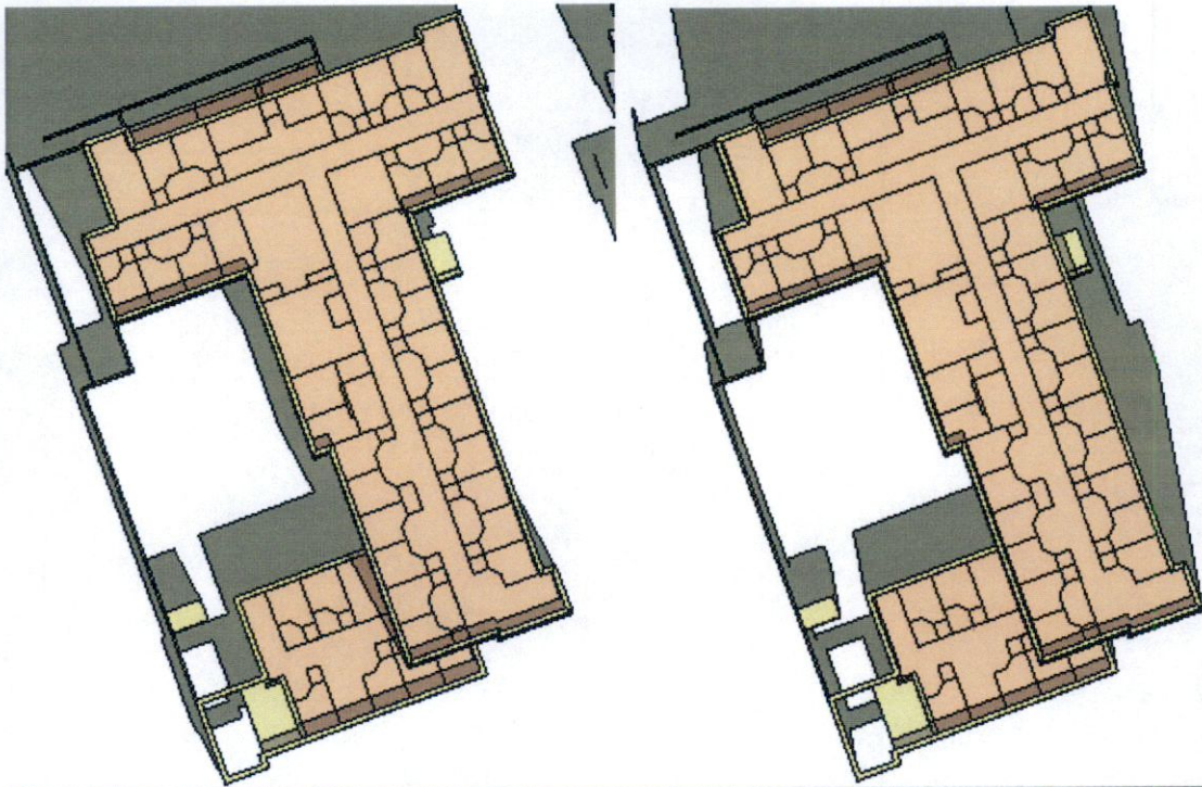
Figure 11: Proposed Site Shadow Analysis on March 21 @11:00 (left) @12:00 (right)
